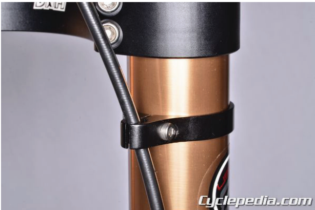
Tighten the hose clamp securely with a 3 mm hex wrench to secure the hose.
