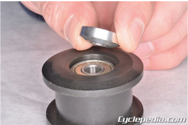
Install the collars on each side of the bearings.
