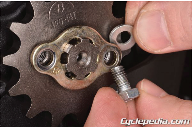
Install the washers between the fixing plate and the sprocket and insert the bolts. Make sure the fixing plate is secure in its groove.
