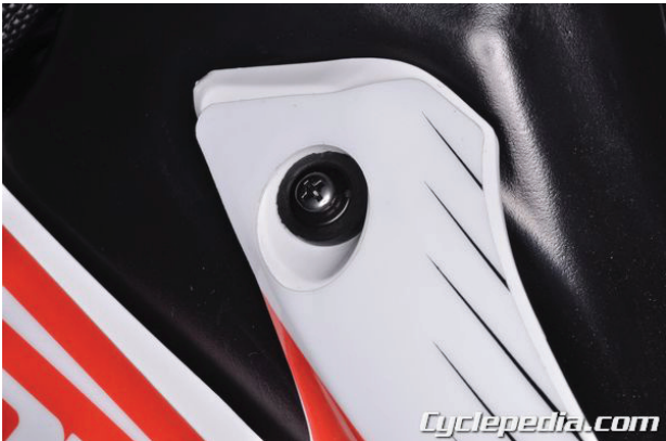
Tighten the upper side cover bolts securely with a #2 Phillips.
