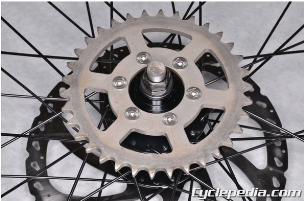
Tighten the rear sprocket bolts to specification with a 5 mm hex socket.
