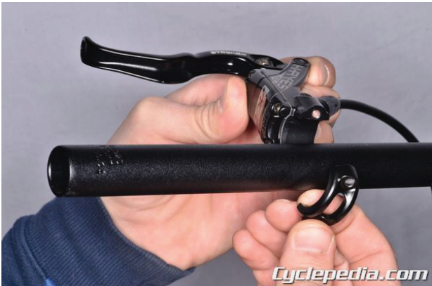
Fit the master cylinder into place on the handlebar.
