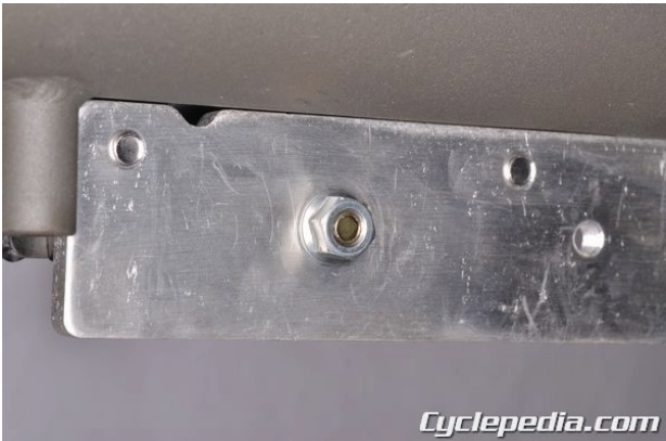
Install the ignition coil nut and tighten it to specification.
