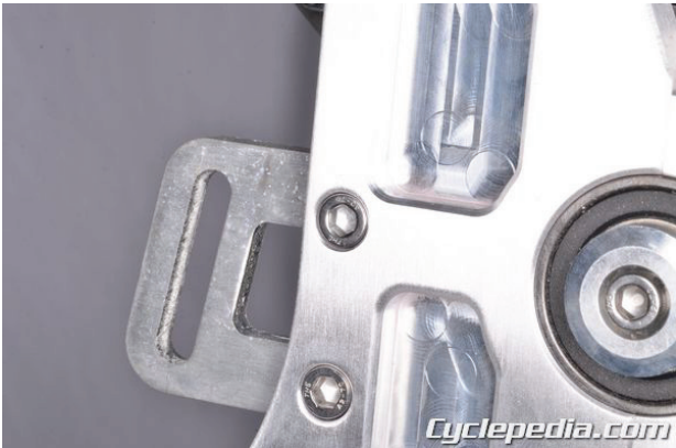
Tighten the drive chain roller/tensioner bracket bolts to specification with a 5 mm hex socket.
