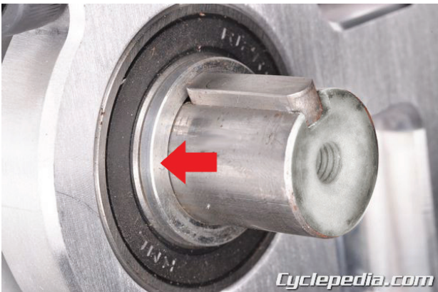
Change the spacer with a thicker or thinner piece to adjust the position of the freewheel sprocket.
