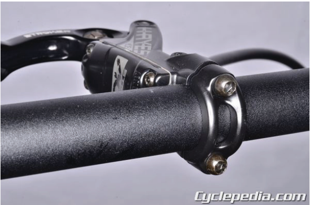
Tighten the clamp bolts evenly so the gap is equal on both sides of the clamp. Tighten the master cylinder to specification with a 4 mm hex wrench
