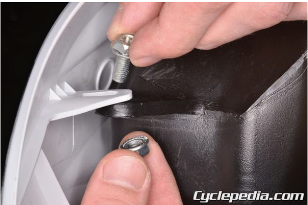
Install the side cover nuts and bolts. Tighten the fasteners securely with a 10 mm wrench and socket.
