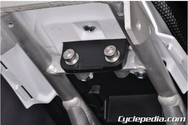
Tighten the seat mounting with a 5 mm hex socket.
