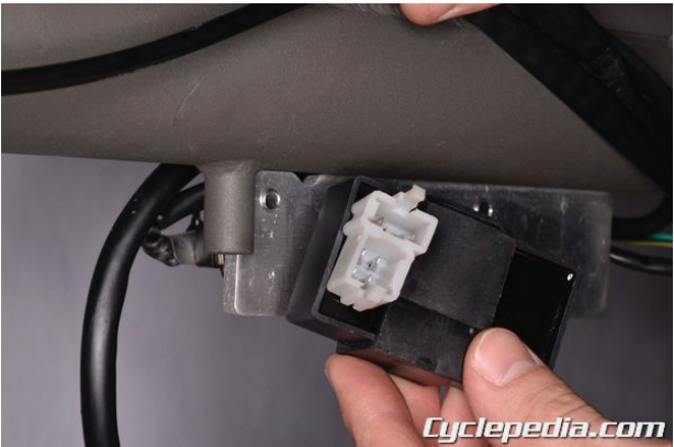
Fit the ignition box into place.
