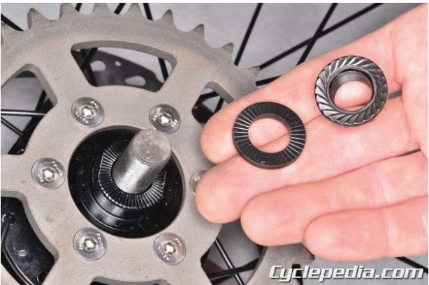
Loosen the rear axle nuts with an 18 mm socket. Remove the axle nuts and washers from the rear axle.
