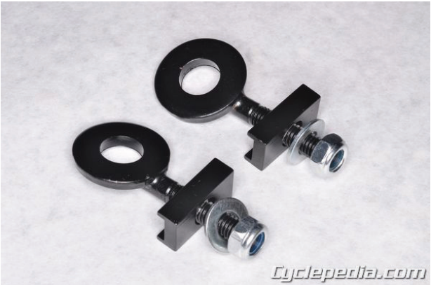
Install the axle tensioners with the rear axle.
