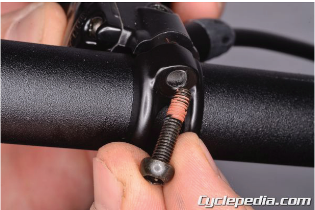
Insert the master cylinder clamp bolts.
