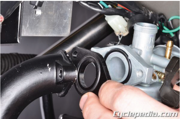
Install the insulator plate so that its O-ring is facing towards the intake manifold.
