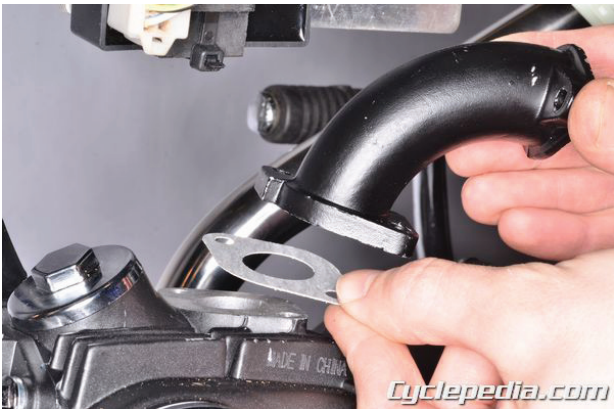
Fit the intake manifold and gasket into place.
