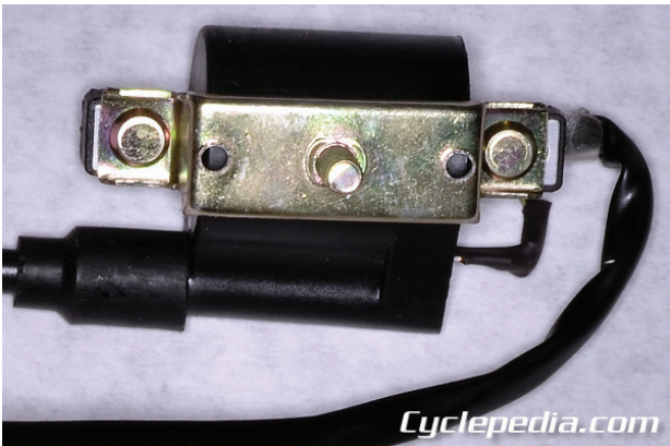
Fit the stud on the ignition coil bracket through the frame.
