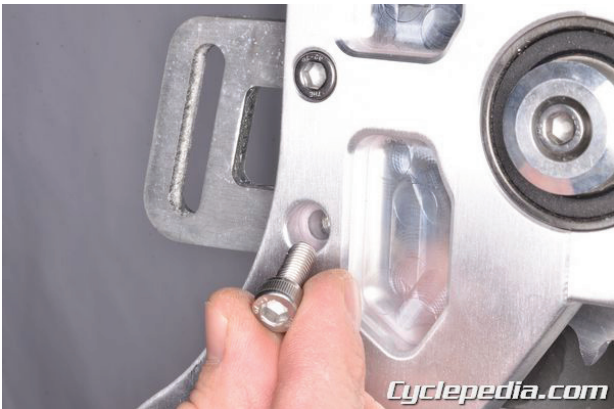
Install the drive chain roller/tensioner bracket mounting bolts.
