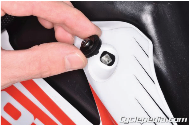
Install the upper side cover bolts and grommets.
