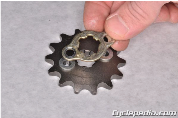
Use washers between the sprocket and fixing plate to adjust the position of the sprocket.
